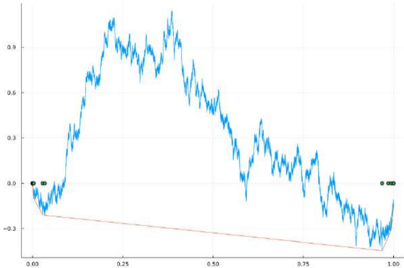
Figure: Path of a Brownian motion on [0, 1] and the convex minorant of its graph.
